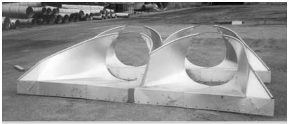
Special fabricated twin end sections.
