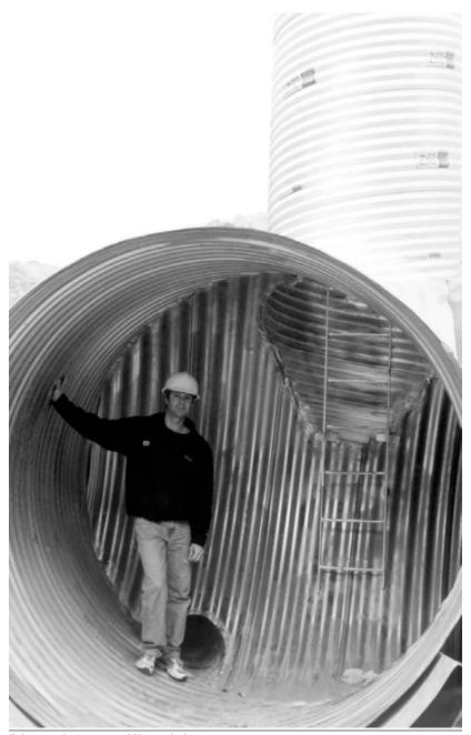
Fabricated riser type CSP manhole.
