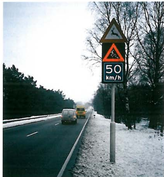
Figure 7.88 - A wildlife warning system combined with heat sensors, used in an area in Switzerland where red deer regularly cross the road. (Photo by H. Bekker)
