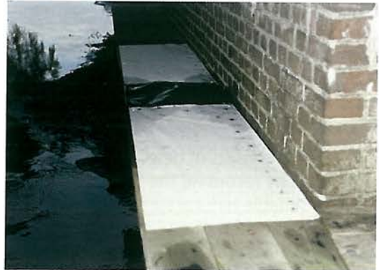
Figure 9.8 - Ink beds are installed on the walkway to allow the passage of small animals such as rodents, shrews or small carnivores to be recorded. (Photo by H. Bekker)
