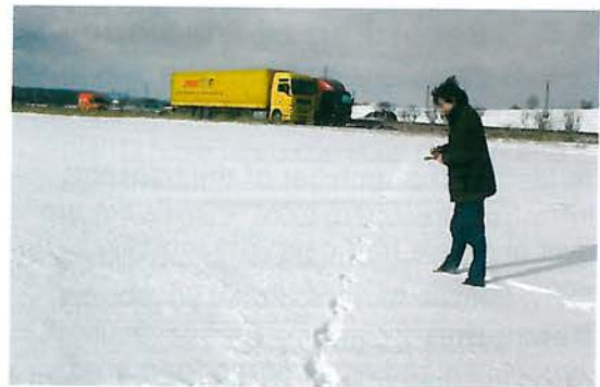
Figure 9.6 - Tracks in the snow allow the number of animals that cross or refuse to cross the infrastructure to be analysed. The method can also be applied to monitor the use of fauna passages. (Photo by V. Hlaváč)
