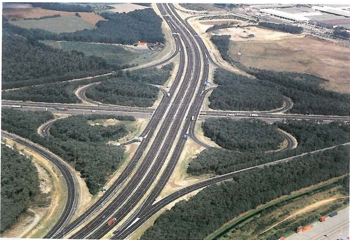
Figure 6.6 - A73, Limburg, The Netherlands. The interchanges have been densely planted to minimise the degree of fragmentation caused to the woodland. (Photo by Rijkswaterstaat, Netherlands)
