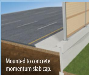
Mounted to concrete momentum slab cap.
