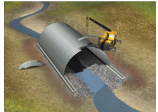
Plates then attach individually to make up other arch segments.
