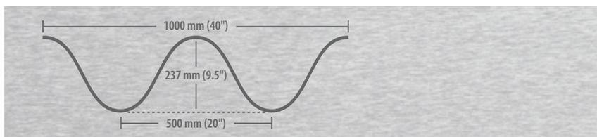
With an impressive 500 mm (20") pitch and 237 mm (9.5") depth, its ultra-large corrugations allow it to reach greater spans and withstand the heaviest of loads. And, just like all AIL engineered solutions, Ultra-Cor ships and installs easily with minimal equipment and labour requirements.
