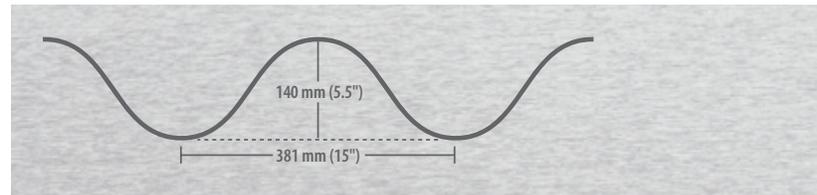
The larger, annular corrugations in Super-Cor® provide nine times the stiffness of conventional structural plate, allowing it to withstand the heaviest of loads. Not only is Super-Cor® the most versatile and economical corrugation on the market, it is also the most internationally-accepted and widely-used.
