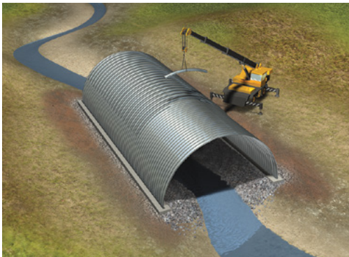
If specified, reinforcement ribs are then added.
