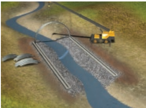
Then, it is lifted into place and bolted to the footings on either side.
