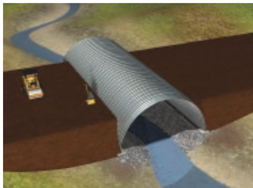
Layers of engineered backfill are added in sequential lifts.
