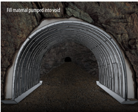
Structures can be advanced to unsupported areas
