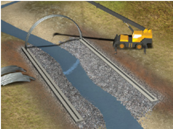
It is then lifted into place and bolted to the footings on either side. In most cases, a boom truck is sufficient for this.
