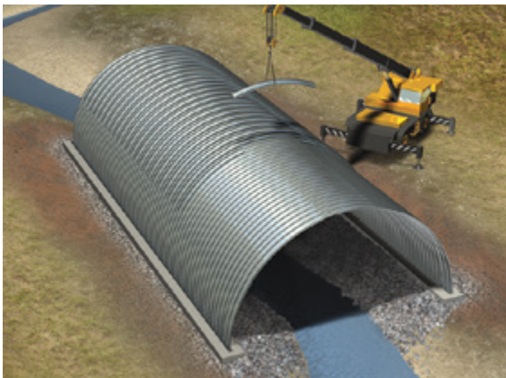
If specified, reinforcement ribs are then added.
