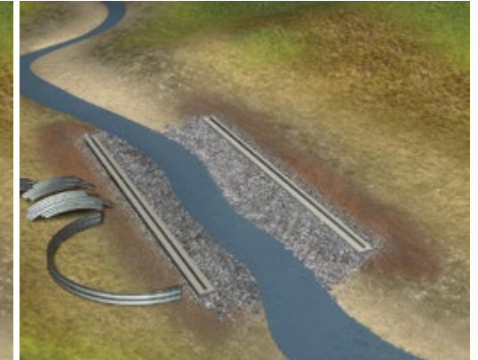
The first arch segment is completely assembled on the ground.
