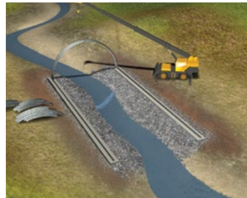
It is then lifted into place and bolted to the footings on either side. In most cases, a boom truck is sufficient for this.
