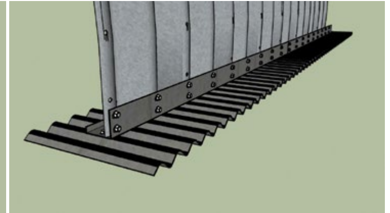
Corrugated Steel Footing
