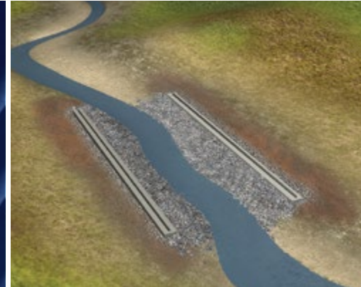
Precast or cast-in-place concrete footings are set over the prepared site.
