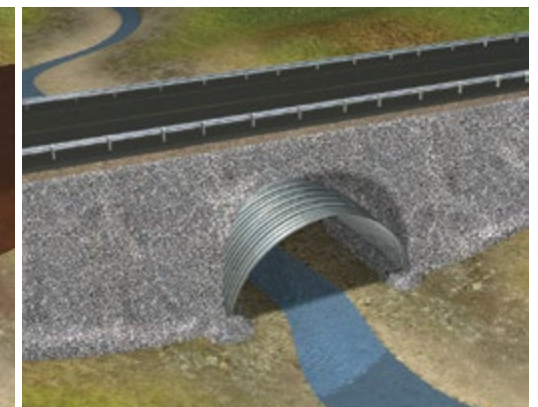
The road surface is then completed with safety barriers.
